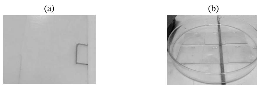
Figure 4. (a) ITO patterning to etch ITO for the contact (b) ITO etching by HCl for 30 min
