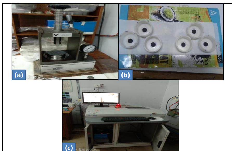
Figure 1: An overview of estimation of trace element (a) Tabletop palletizer, (b) Pellets in a mould cups, (c) EDXRF-3600 Spectrometer
