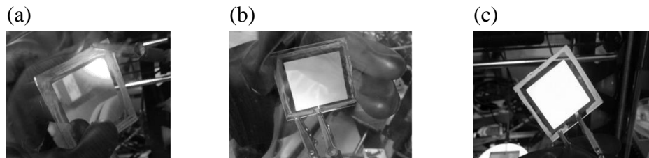
Figure 8(a) Malfunctioning blue OLED sample (b) Unevenly lit red OLED sample and (c) Super yellow OLED sample with small inconsistencies
